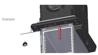
Fixing by means of profile in the door groove
