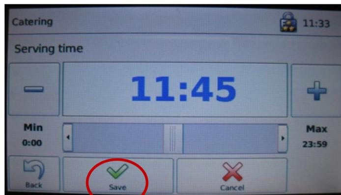
➤ Set the time using the **slider** or the **+ - keys**.
