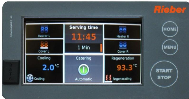
The controllable functional units can be freely programmed. This can be done directly on the control panel. Parameters and measuring data can be transferred via USB stick.
